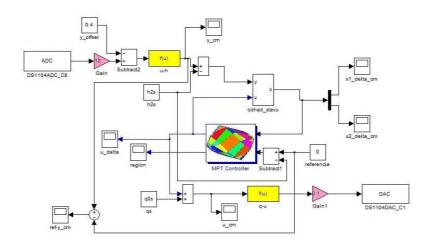
Figure 2: Simulink scheme for real-time experiments.
