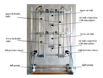
Figure 1: The laboratory liquid tanks equipment.
