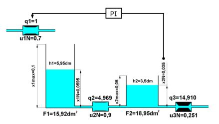
*Figure 1: Two tank system with PI controller*
