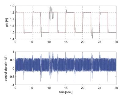
Figure 11. Response of controlled system with no friction compensation
