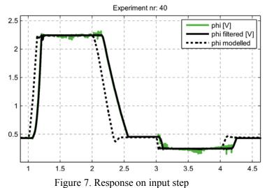
Further, two dynamic parameters J and b must be determined. We have used the step response of the system shown in Fig. 7. One can see that there is still some unmodelled dynamics causing time delay in the system.
