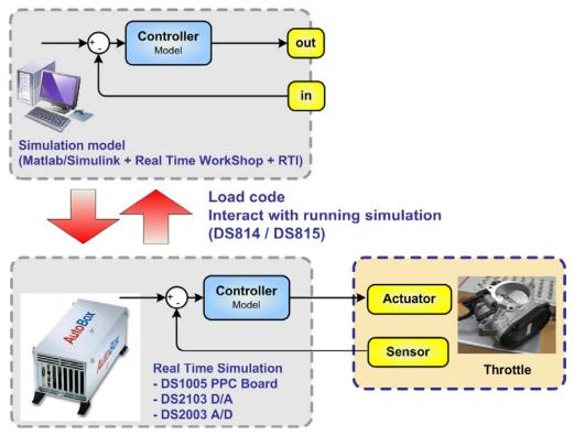
Figure 8: Principal schematic of RCP
