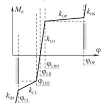
Figure 3. Schema of nonlinear spring (LH – limp home, CL – throttle closed, OP – throttle opened)
