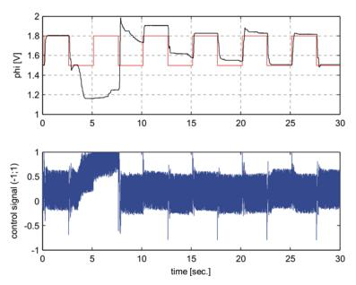
Figure 12. Response of controlled system after the manual disturbance of valve position
