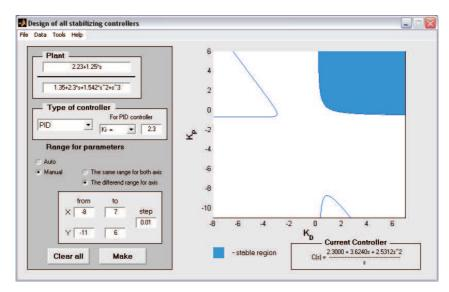
Figure 2: GUI for design of stabilizing controllers
