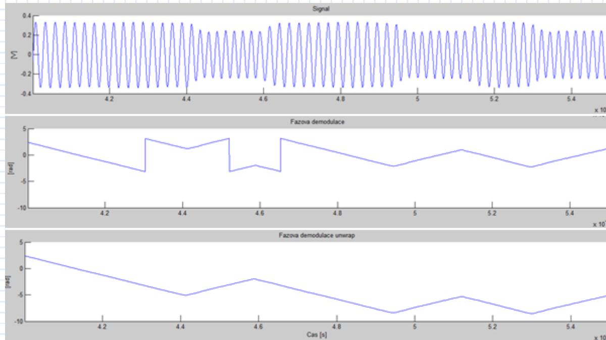
$$f = \frac{\omega_1 - \omega_2}{2\pi(t_1 - t_2)} + f_{stř}$$
