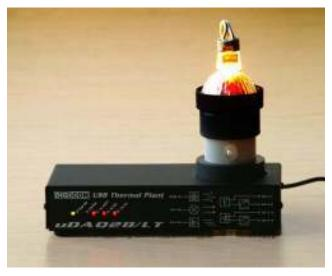
Figure 2: Thermo-optical plant
