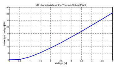
Figure 3: I/O characteristic of the thermo-optical plant
