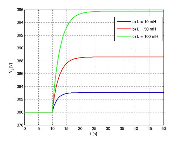
Figure 6: The terminal voltage of synchronous generator response to the step change of excitation voltage
