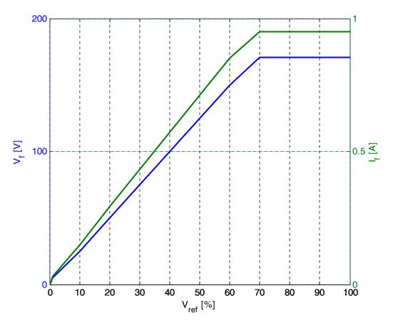
Figure 4: The excitation current and excitation voltage limit
