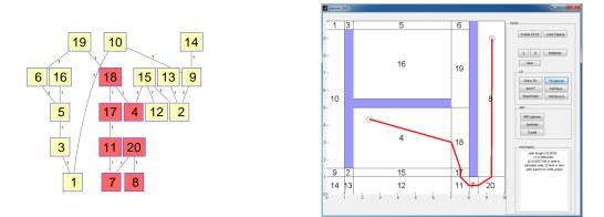
Figure 7: Cell-decomposition planner GUI and generated graph.
