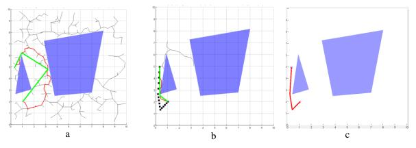
Figure 8: RRT planner without /with bias to Cell-decomposition points and Cell-decomposition path
