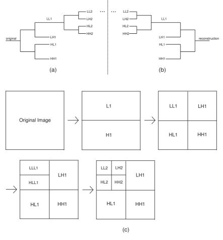
Figure 1: 2D DWT decomposition into two levels: (a) Image decomposition, (b) Image reconstruction, (c) Scheme of decomposition up to the second level
