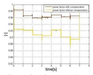
Fig. 5 – The course of power factor with and without compensation
