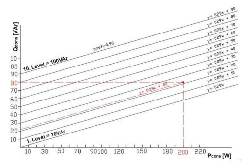
Fig. 3– the controller principle – comparison of lines displacement on the y-axis (desired value of power factor is 0,96)
