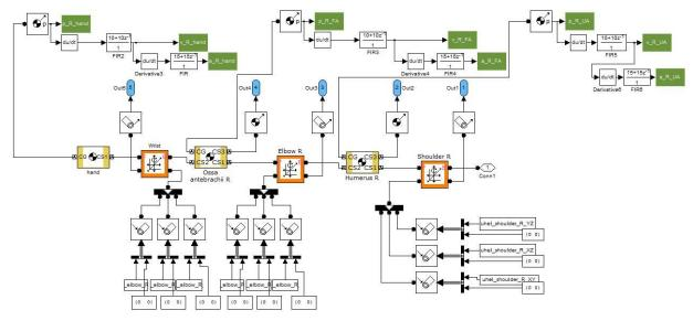
Figure 4: Model of right human arm created in Simulink workspace.
