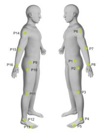
Figure 1: Draft position of the markers on the body for physiotherapeutic examination by 3D Lukotronic AS 200.
