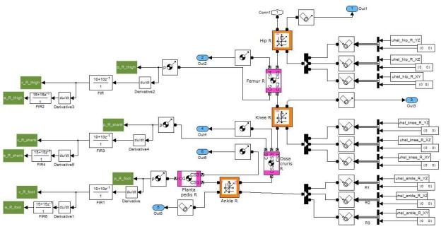
Figure 5: Model of right human leg created in Simulink workspace.
