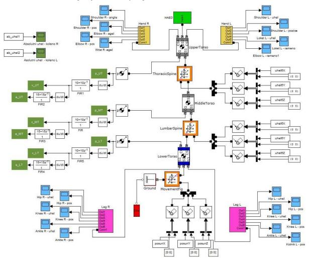
Figure 3: Model of human body created by Simulink workspace.
