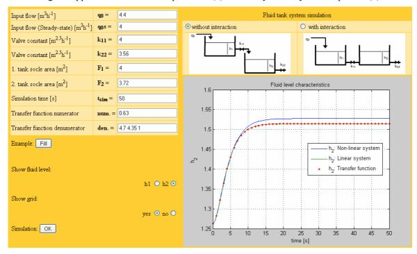
Fig. 3: Storage tank system simulation
