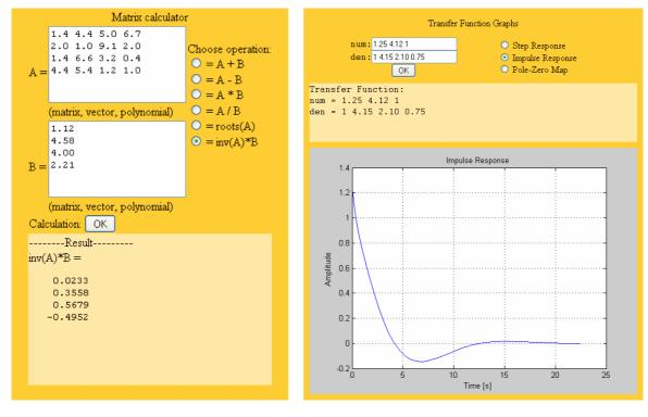
Fig. 2: Applications for matrix operations (a) and for dynamic system responses (b)
