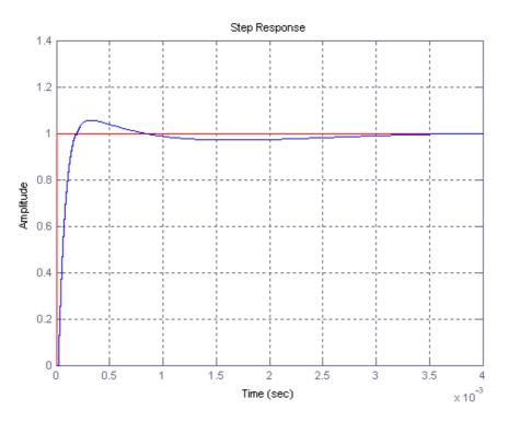
Figure 5: Result of simulation response regulated system to step response
