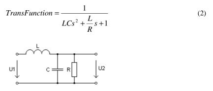
Figure 3: Controlled circuit
