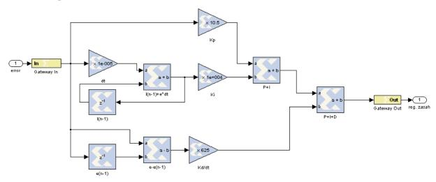
Figure1: PID controller built from System Generator blocks
