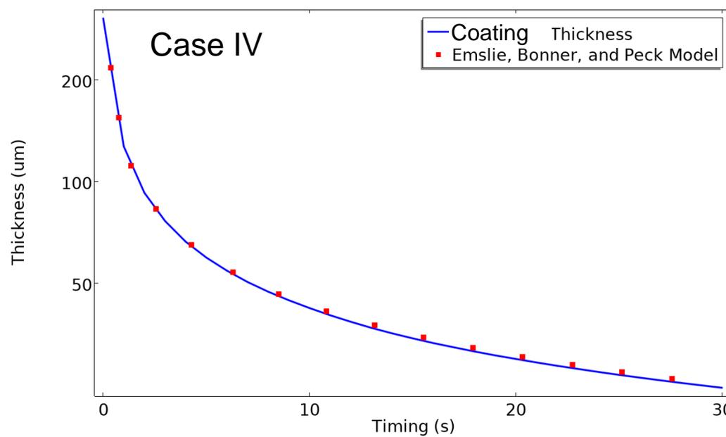
As the substrate rotates, the solution is thrown out from all around, and the thickness of the coating layer gradually becomes thinner
