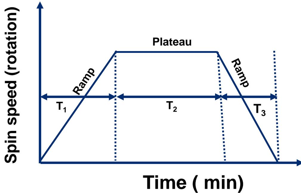
A spin profile with steep ramps (short T1 and T3), and an adjustable short plateau (T2) to attain thicker and at the same time, more homogeneous films.
