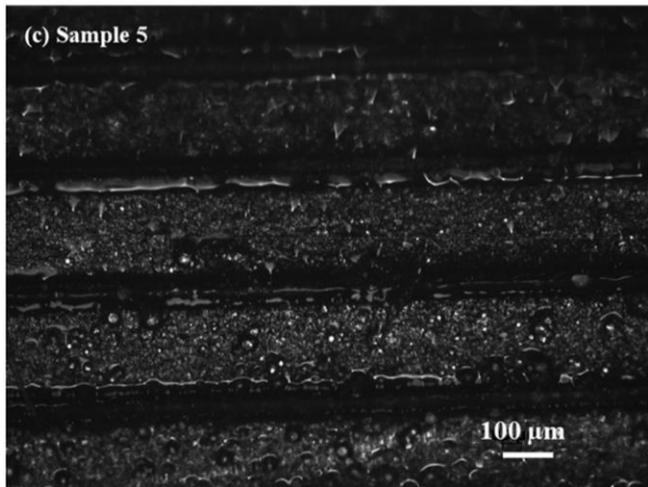
**(a) PMMA coating on NiTi surface (b) PMMA coating with some pin hole on the top surface (c) NiTi surface through a transparent layer of PMMA coating (4.2 mol. %), 500 rpm.**
