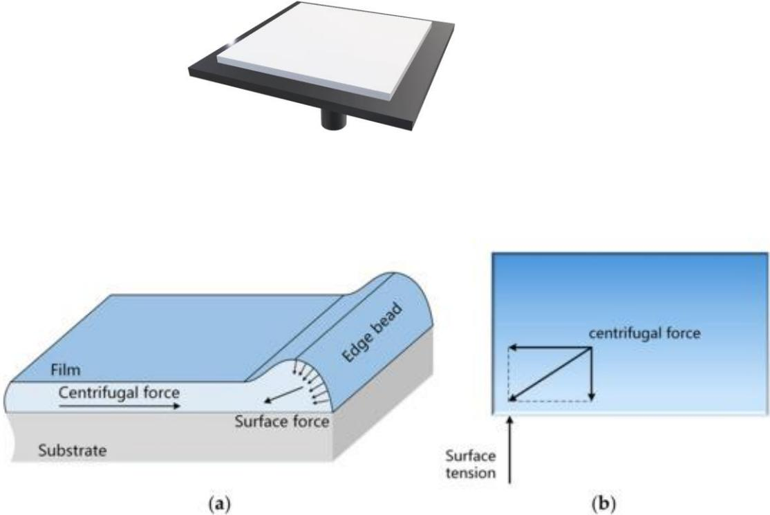
The thinning of a Newtonian, volatile liquid film of thickness  $h$  on a rotating support is described by Meyerhofer
