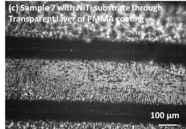
**PMMA coated NiTi surface with laser lines at 4.2 mol % at RT**
