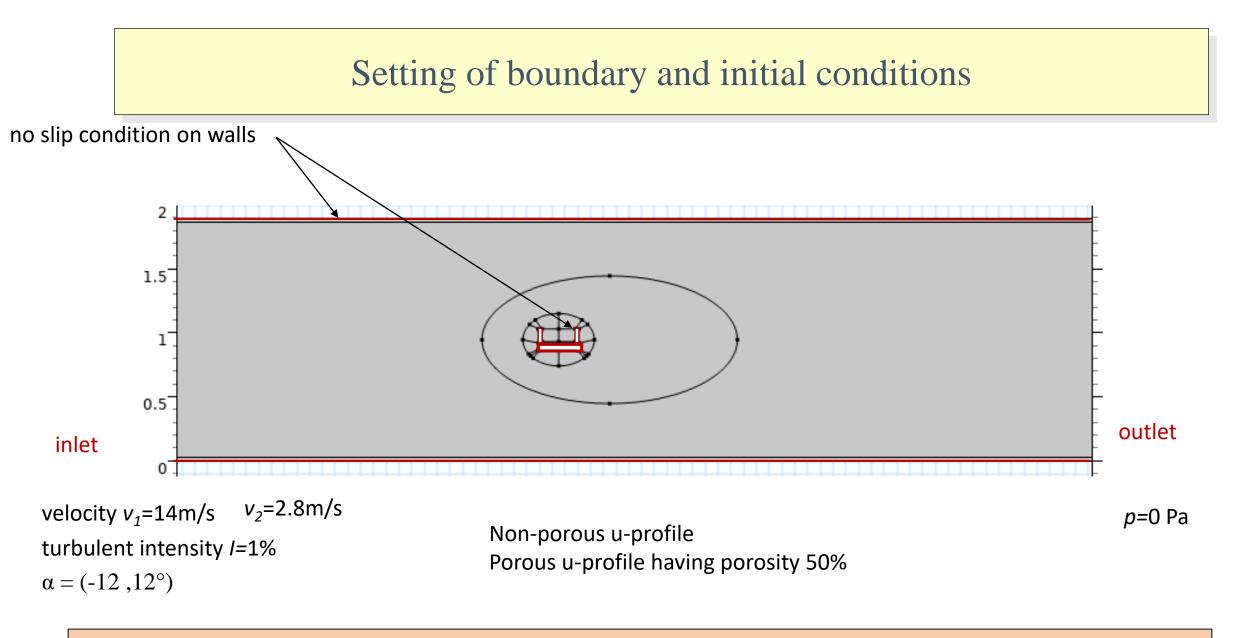
=> evaluation of mean drag and lift coefficient, fluctuating lift coefficient, Strouhal number and flow characteristics
