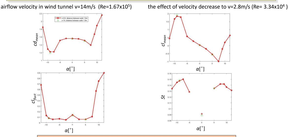
aerodynamic characteristics do not change markedly with the change of inlet velocity =>  $v_2$ =2.8m/s used in further calculations
