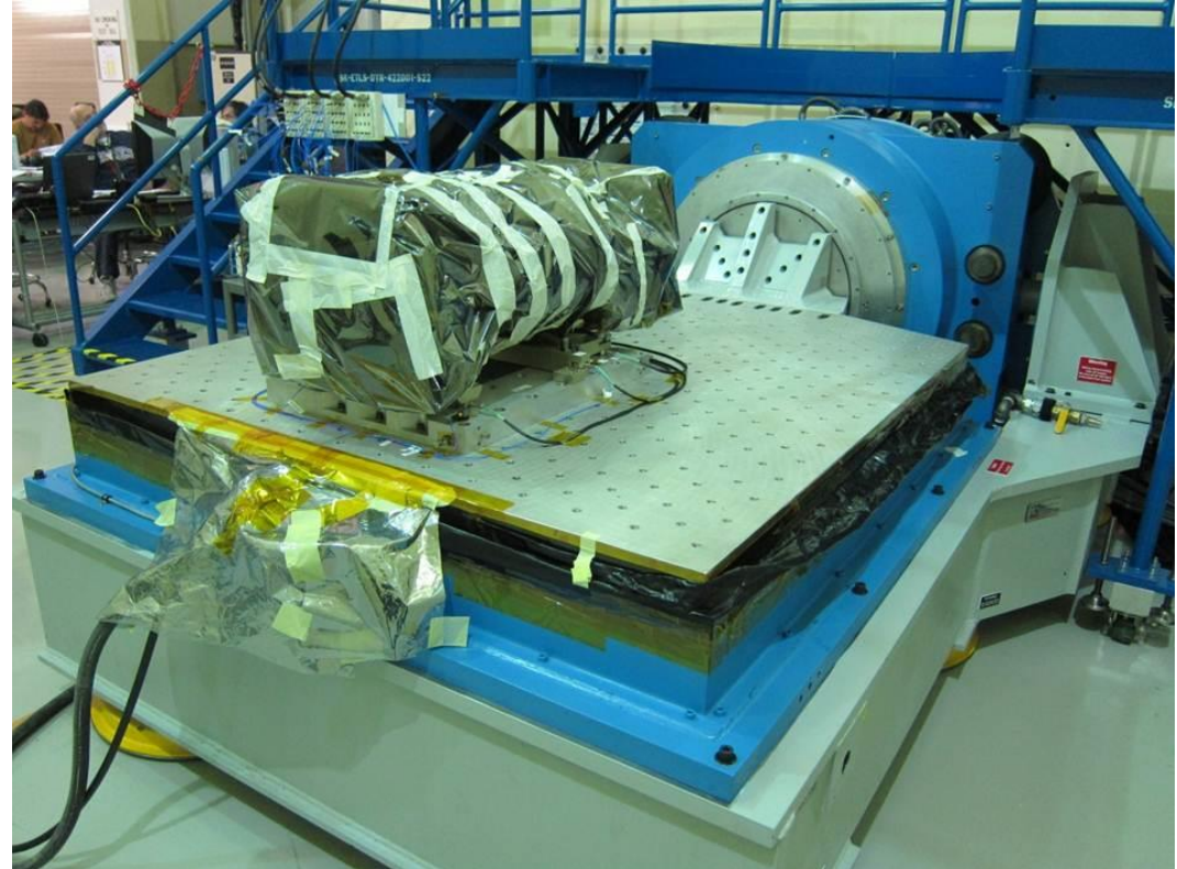
GOES-R SUVI Undergoes Vibration Testing
